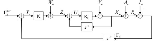
Fig. 3. Linearized Power Control Loop
