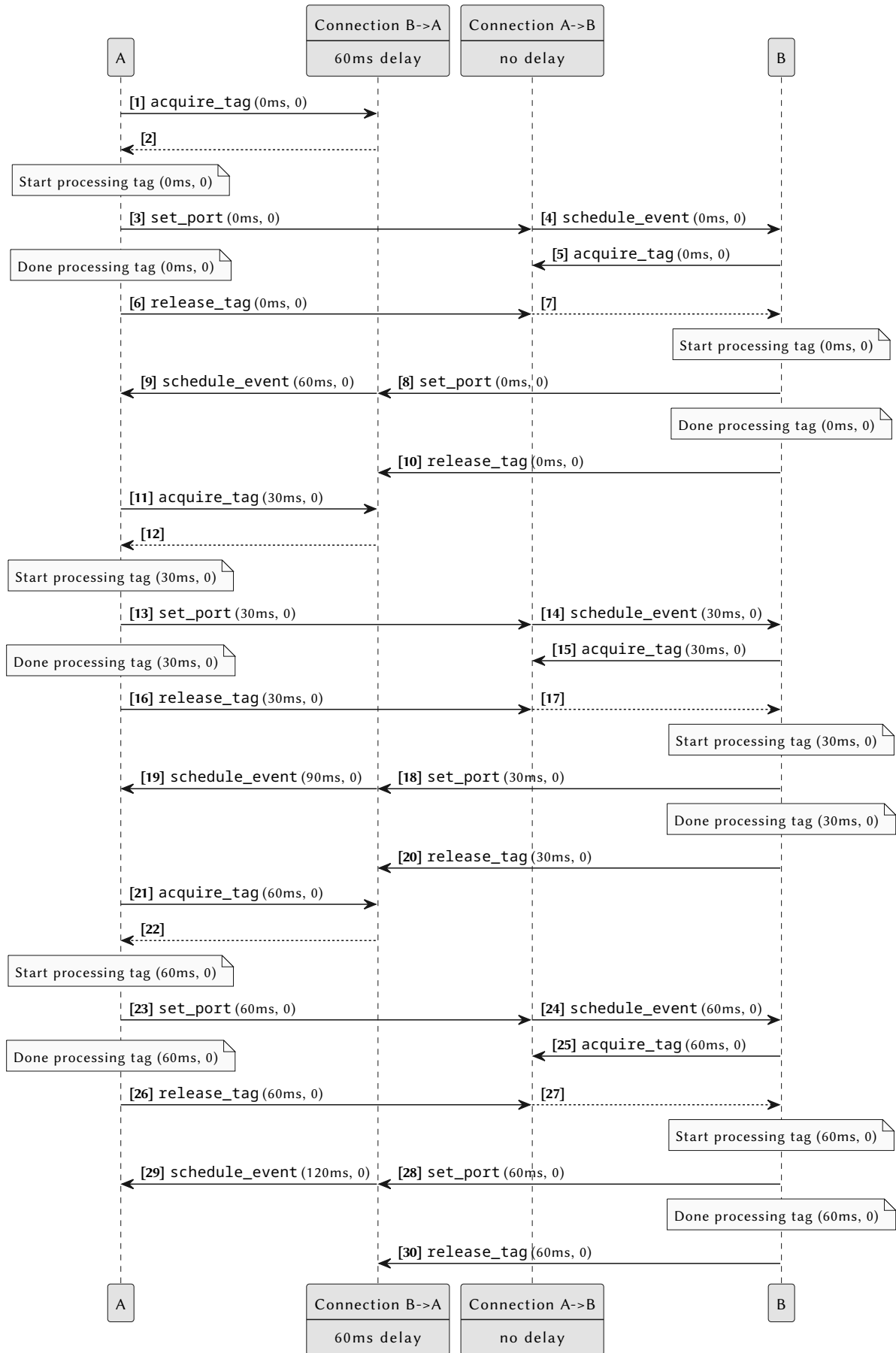
Figure 6.22: A sequence diagram that shows the communication between A and B for the program in Figure 6.21.
