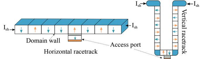
Fig. 1: Horizontal and vertical configurations of DWM.
