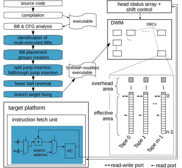
Fig. 3: Overall flow, supporting hardware and DWM structure associated with SHRIMP. Contributions of this work highlighted.
