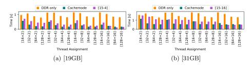
Fig. 1: Comparison of cases 1,2 and 3. X-axis [X+Y] shows X = threads assigned to MCDRAM and Y = threads assigned to DRAM
