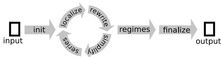
Figure 5.4.: Herbie's process for improving program accuracy [Pan+15, Figure 1].
