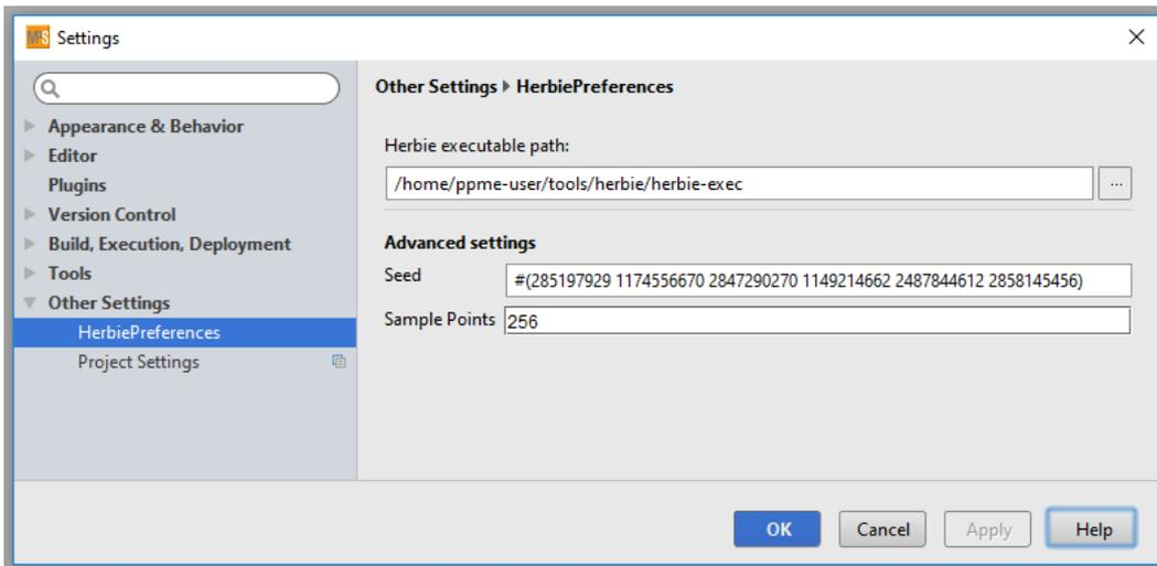
Figure 5.5.: Configuration panel for the Herbie integration in PPME.
