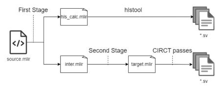
Figure 4.1: FPGA Backend Workflow
