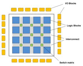
Figure 2.3: FPGA Architecture [BP21]
