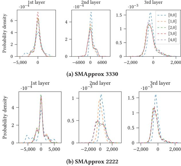
**Figure 4: Error distributions on first neurons on 1st-3rd layers of ALL-CNN. Labels indicate the neuron position in the 1st channel of the output tensor.**
