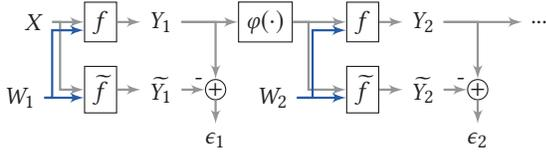
Figure 2: Approximation error measurement on a DNN
