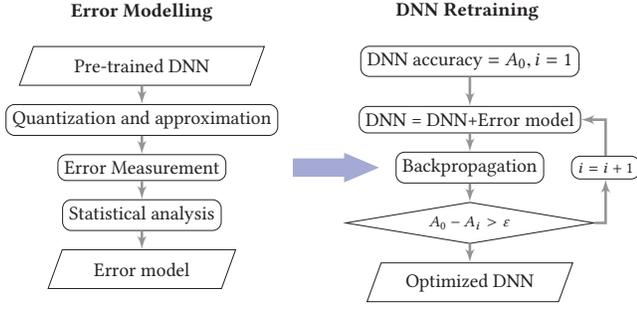
Figure 1: Modelling the Approximation Error in DNNs
