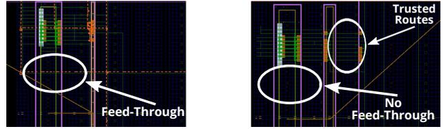
Fig. 5: The final result of AMAH-Flex on UltraScale+. *Left*, an example of a feed-through as an orange colored dashed arrow (without AMAH-Flex or without IDF). *Right*, using trusted routes and free of feed-throughs (using AMAH-Flex).
