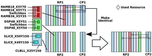
Fig. 4: Example of the result of our *make identical* algorithm on Xilinx Virtex7.
