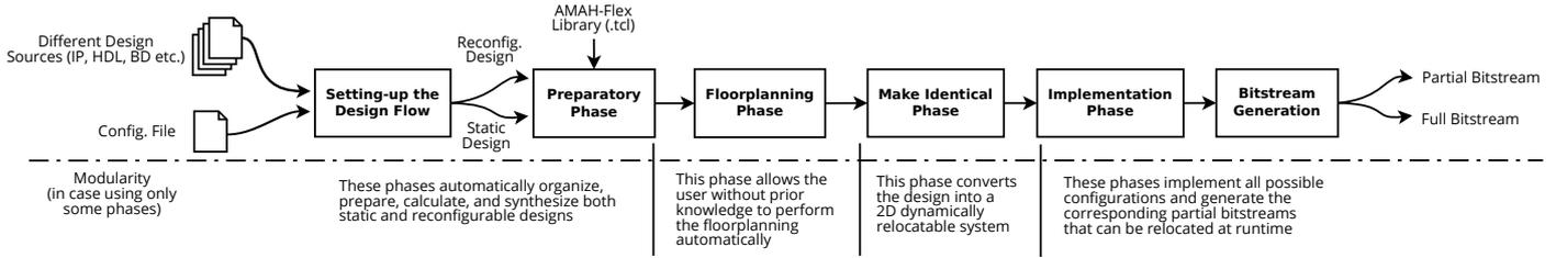
Fig. 1: On the upper half a general overview of the design flow of our tool and its phases. On the bottom page, a general description of modularity, in case the subphases are used separately.
