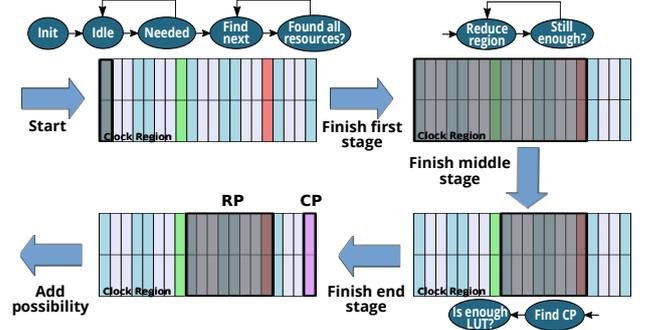
Fig. 3: A detailed overview of the *find possibilities* procedure including the three stages and their states. Example of a placing possibility: 3 CLB columns (blue) and 1 DSP column (red). Gray are the interconnections.
