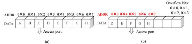
Fig. 4. Example of racetrack as shift register: (a) initial status; (b) after accessing the position  $0 \times 5$ .
