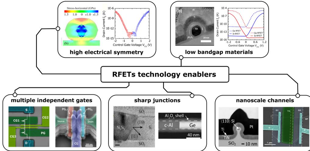
Figure 3: Summary and visual exemplification of the five main technology enablers for successful RFET device fabrication, as discussed in the text.
