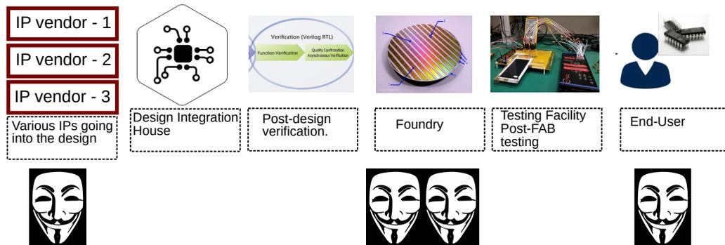
Figure 7: Security from the perspective of global IC supply chain. Most vulnerable points are IP-vendors, foundry and the end-users. Of these, foundry is the most vulnerable point as various attack measures such as counterfeiting, over-production, insertion of hardware Trojans etc. can be realized.
