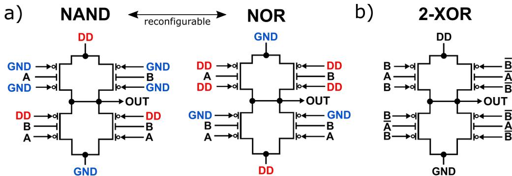
Figure 4: Comparison of explicit and implicit reconfigurability on the logic gate level on the example of (a) a reconfigurable NAND/NOR gate and (b) an compact functional-enhanced XOR gate.
