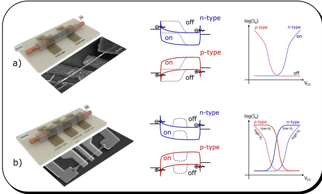
Figure 1: Schematics, SEM images, band diagrams, and generic transfer characteristics of Schottky barrier based nanowire RFET. (a) Dual gated RFET with individual control at each barrier and (b) three-gated RFET with programming at both junctions simultaneously are shown.
