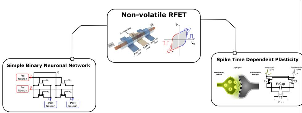
Figure 8: Neuromorphic Computing with RFETs. (a) Schematic of a three-gated RFET with added non-volatile storage option by placing a ferroelectric material within the gate dielectric as enabler for neuromorphic circuit designs. (b) circuit diagram of a simple Binary Neuronal Network realized by RFETs (c) circuit diagram of a synapse able to realized spike-time-dependent-plasticity. (d) Generic representation of a biological synapse.
