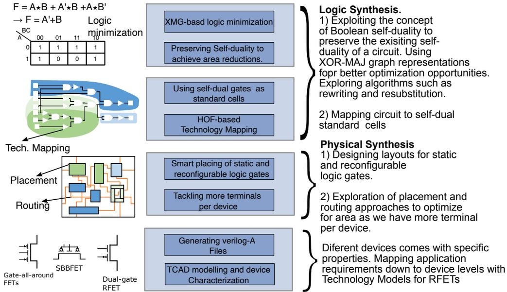
Figure 5: Capable EDA flows are imperative for the overall development of RFET technology. This requires exploring techniques and approaches that can exploit their unique properties. We list down recent proposed approaches developed specifically for RFETs.
