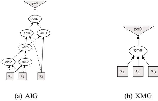
Fig. 1: Edges and nodes representation in case of AIG and XMG representation for the function,  $f = x_1 \oplus x_2 \oplus x_3$  (3-input XOR). The AIG has 6 gates and 13 edges, while the XMG has 1 gate and 4 edges.
