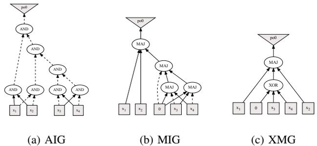
Fig. 5: Different logic representations of the function,  $f = \langle x_1, x_2, (x_3 \oplus x_4) \rangle$ . One can notice that the number of nodes and edges are the lowest in the XMG representation.
