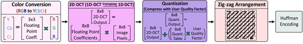
Fig. 3. Kernel structure of JPEG Compression application.
