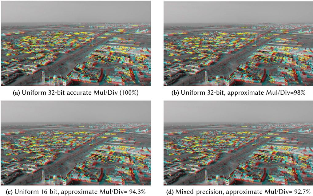
Fig. 15. Corners and vector detected via Harris Corner Detection application: As can be seen even with approximation, the direction of the movement has been found by many vectors.
