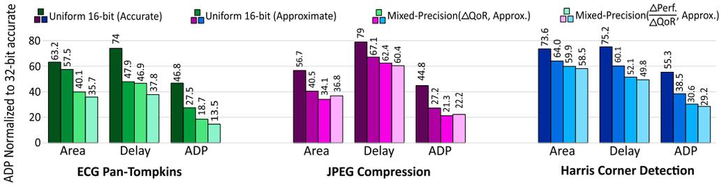
Fig. 12. End-to-end performance gains of different strategies, compared to 32-bit accurate (uniform) configuration: overall, mixed-precision configurations, generated by the proposed  $\frac{\Delta ADP}{\Delta QoR}$ -based heuristic achieves higher gain than the  $\Delta QoR$ -based heuristics [29, 63].
