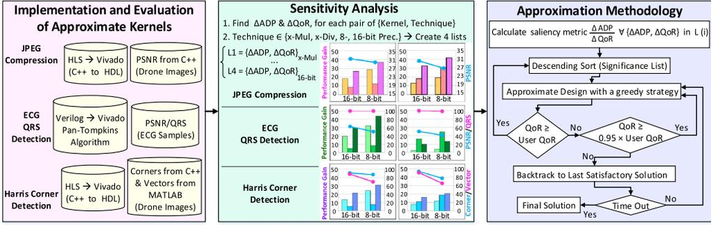
Fig. 7. Overall three-step flow for the proposed sensitivity analysis and cross-layer approximation methodology.
