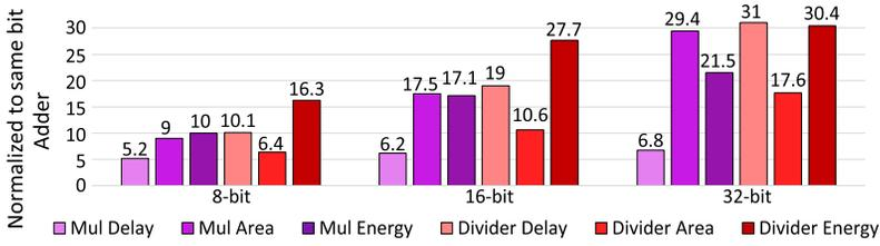
Fig. 1. Comparing area, delay, and energy of 8-, 16-, and 32-bit addition, multiplication, and division operations, when implemented in Virtex-7 FPGA, via Look-up Table (LUT)-based accurate IPs.
