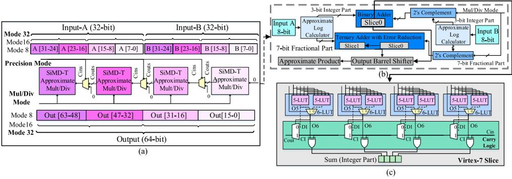
Fig. 5. (a) SIMDive structure, (b) proposed 8-bit multiplier/divider, (c) Virtex-7 slice (used for addition/subtraction of integer/fractional parts).
