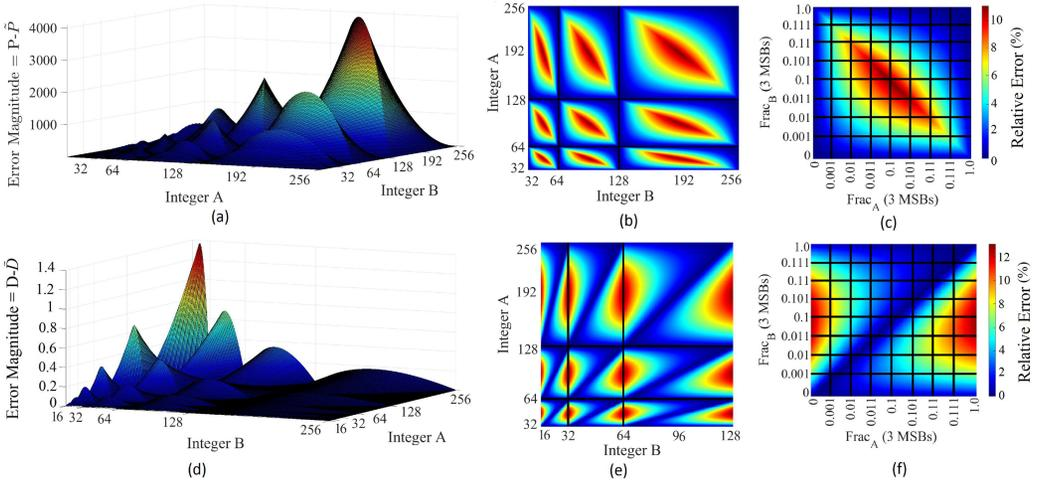
Fig. 6. Mitchell's error:  $8 \times 8$  multiplier (top),  $16/8$  divider (down). Parts (b) and (e) show error repeats the same behavior in each power-of-two interval (i.e., each multiplier or divider size). Parts (c) and (f) show the proposed error-reduction scheme: Dividing squarish zone of fractional-parts to 64 regions, each has a specific coefficient.
