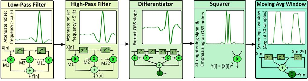
Fig. 2. Kernel structure of Pan-Tompkins QRS detection application.
