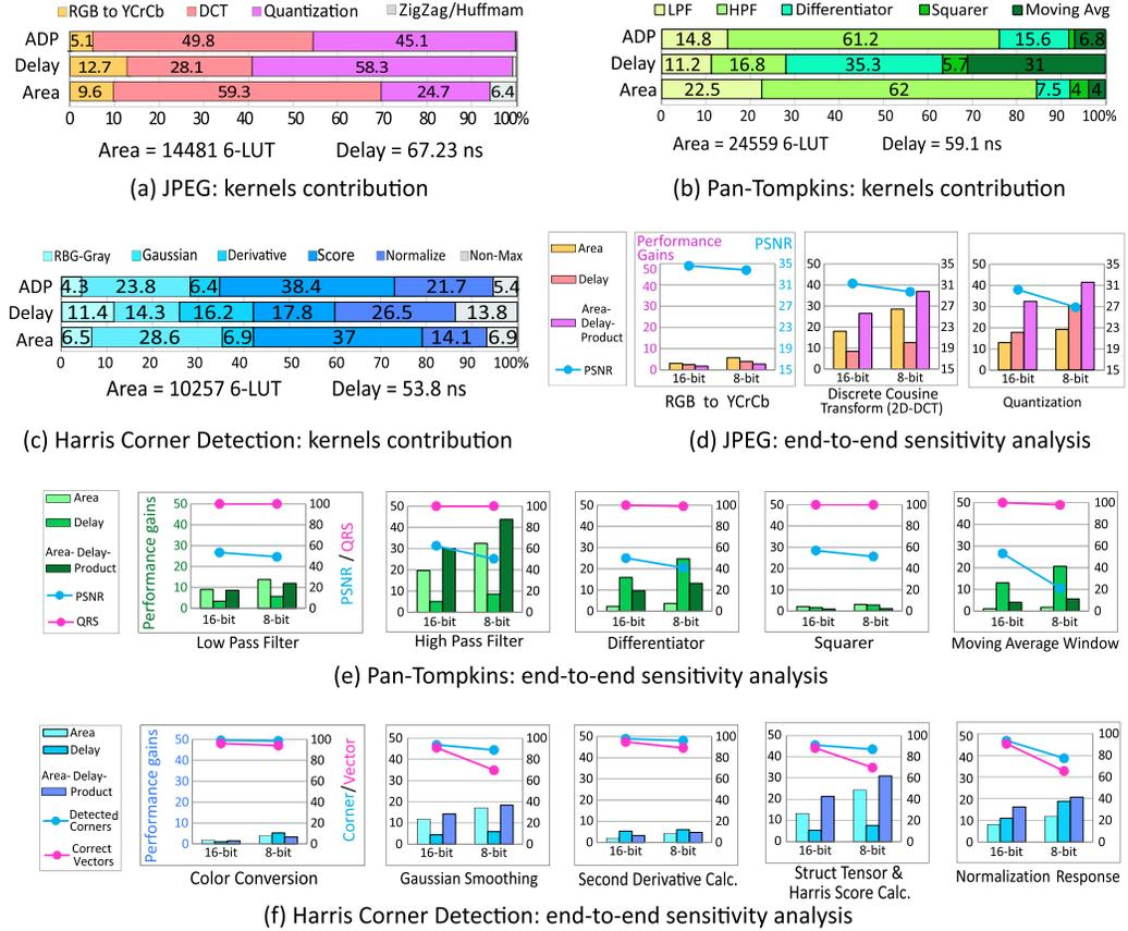
Fig. 8. Sensitivity analysis to cross-layer approximation in three applications. (a), (b), (c): contribution of each kernel in performance metrics of accurate implementation. (d), (e), (f): the tradeoff between end-to-end performance gains and QoR degradation after scaling down the precision of *one* kernel having SIMDive Mul/Div, while the rest are 32-bit accurate (32-bit integer with accurate operations). Area is in terms of LUT and delay in terms of ns.
