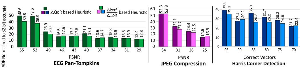
Fig. 13. Comparing  $\frac{\Delta ADP}{\Delta QoR}$ -based versus  $\Delta QoR$ -based heuristic in various QoR levels: The former approach has generated configurations with higher ADP improvement when the accuracy threshold is high.
