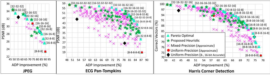
Fig. 11. *Approximate, mixed-precision* configs generate accuracy-performance tradeoffs with similar/higher gains than *accurate-uniform*. The heuristic also finds many of Pareto/near-Pareto points. Configs found in 20% of exhaustive time are distinguished by green stars (QoR thresholds: JPEG 28 dB, ECG 35 dB, HCD 90%).
