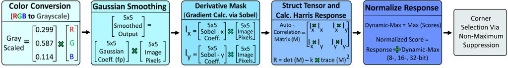
Fig. 4. Kernel structure of Harris Corner Detection application.
