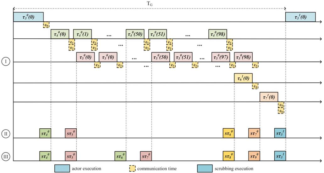
Fig. 11. (I) *h.263* encoder SDFG schedule. (II) Proposed scrubbing execution for  $\Upsilon = 11\text{ms}$ . (III) Proposed scrubbing execution for  $\Upsilon = 4.13\text{ms}$ .
