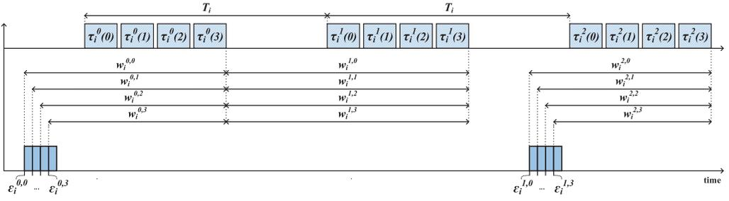
Fig. 6. Time interval between last scrubbing process, in particular the frame  $f$ , and the beginning of the  $l^{\text{th}}$  user task execution on the iteration periods 0 and 1.
