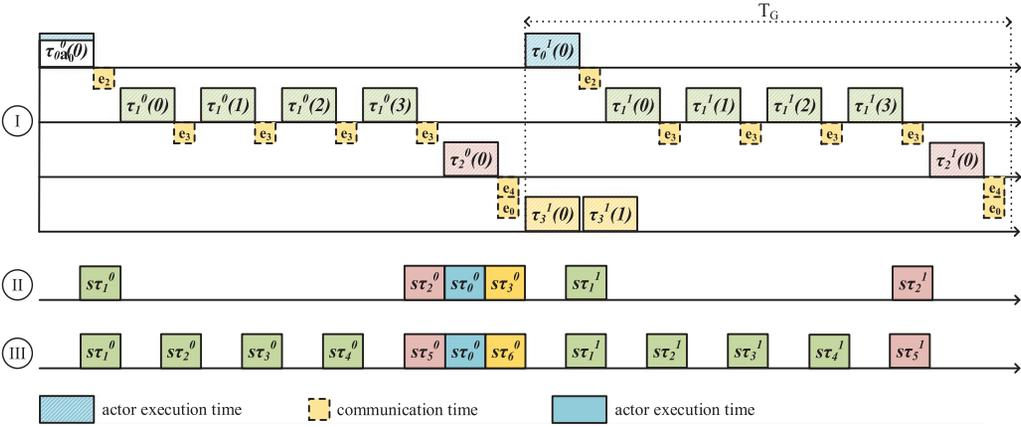
Fig. 7. Scrubbing execution. (I) User task execution example. (II) Scrubbing execution: Only one scrubbing task associated with each user task. (III) Scrubbing execution: More than one scrubbing task can be associated with one user task according to their execution behavior.
