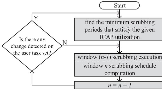
Fig. 8. Scrubbing schedule window mechanism—flowchart.
