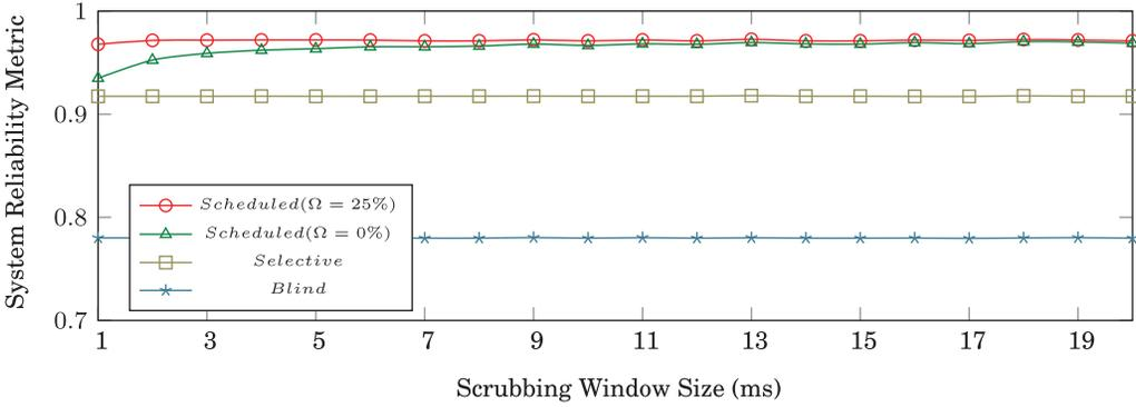
Fig. 14. System reliability metric over the scrubbing schedule window size. Criticality is assigned according to the user criteria ( $cu$ ). All the user applications have the same criticality in this experiment.
