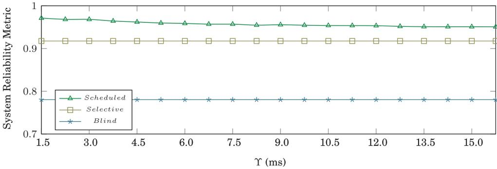
Fig. 12. System reliability metric over  $\Upsilon$ . Criticality is assigned according to the user criteria ( $cu$ ). All the user applications have the same criticality in this experiment.
