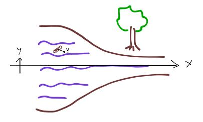
Consider a river that is flowing through a narrowing channel. Flow is steady and does not change with time, and the river shore is far away from the origin of our coordinate system. Flow at position (x, y) is specified by:
