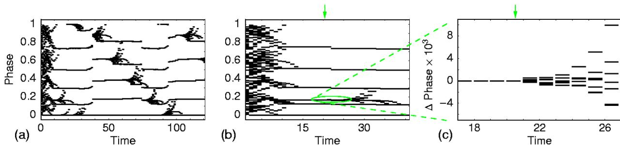
Figure 1: Phase dynamics of a large network ( $N = 100$ ,  $\varepsilon = 0.2$ ,  $\tau = 0.15$ ). Phases of all oscillators are plotted whenever a reference oscillator has been reset. (a) Dynamics with noise ( $\eta = 10^{-3}$ ), (b) deterministic dynamics in response to a single phase perturbation (arrow,  $\sigma = 10^{-3}$ ), note that the system switches from a six-cluster to a five-cluster state, (c) phase differences evolution.
