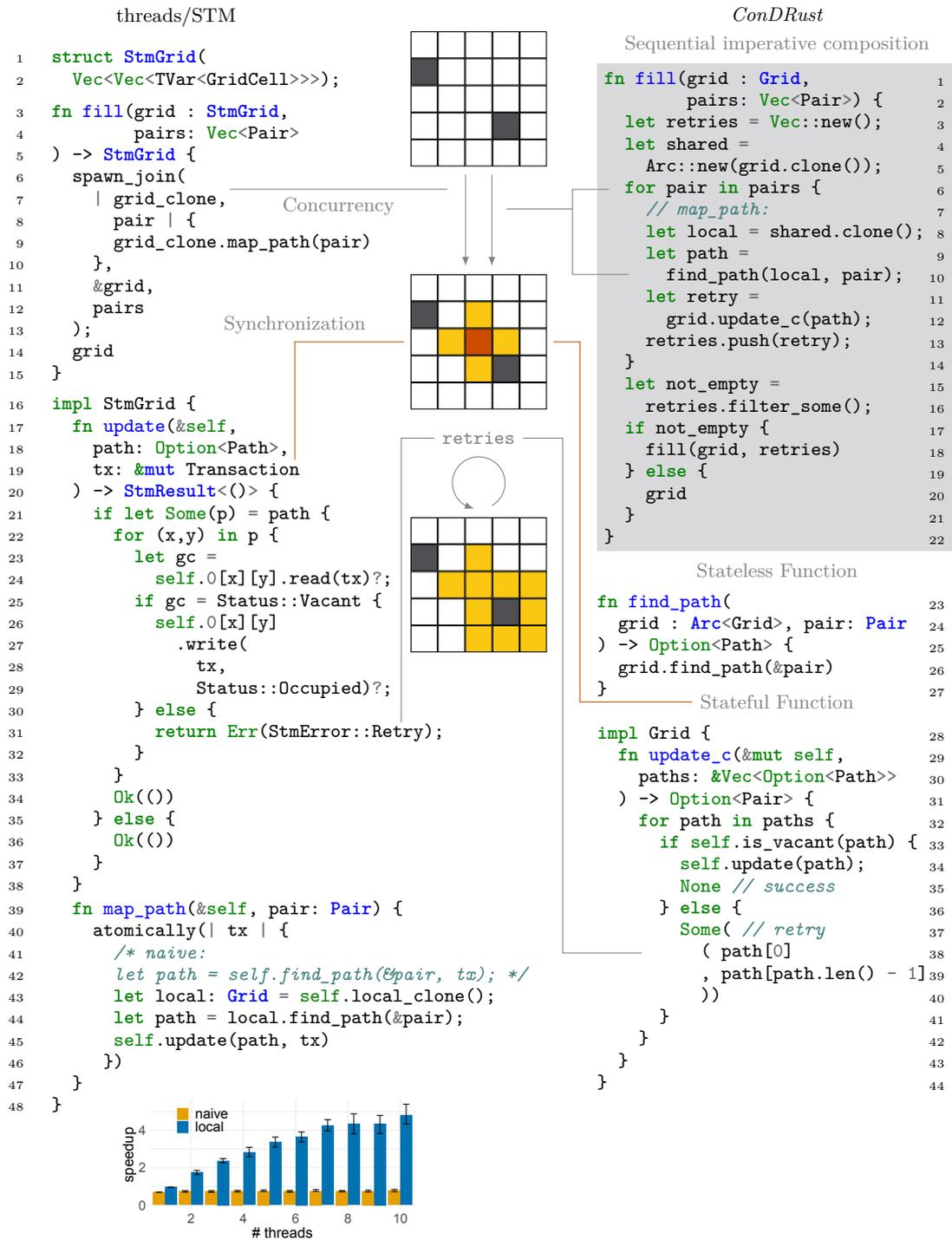
■ **Figure 4** Introducing concurrency into the labyrinth benchmark adds collisions. The left column shows the implementation with threads and STM. The right column shows the imperative sequential *ConDRust* program.
