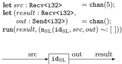
■ **Figure 12** A  $\text{Ⓜ}_p$  program with a single identity node and the corresponding dataflow graph.
