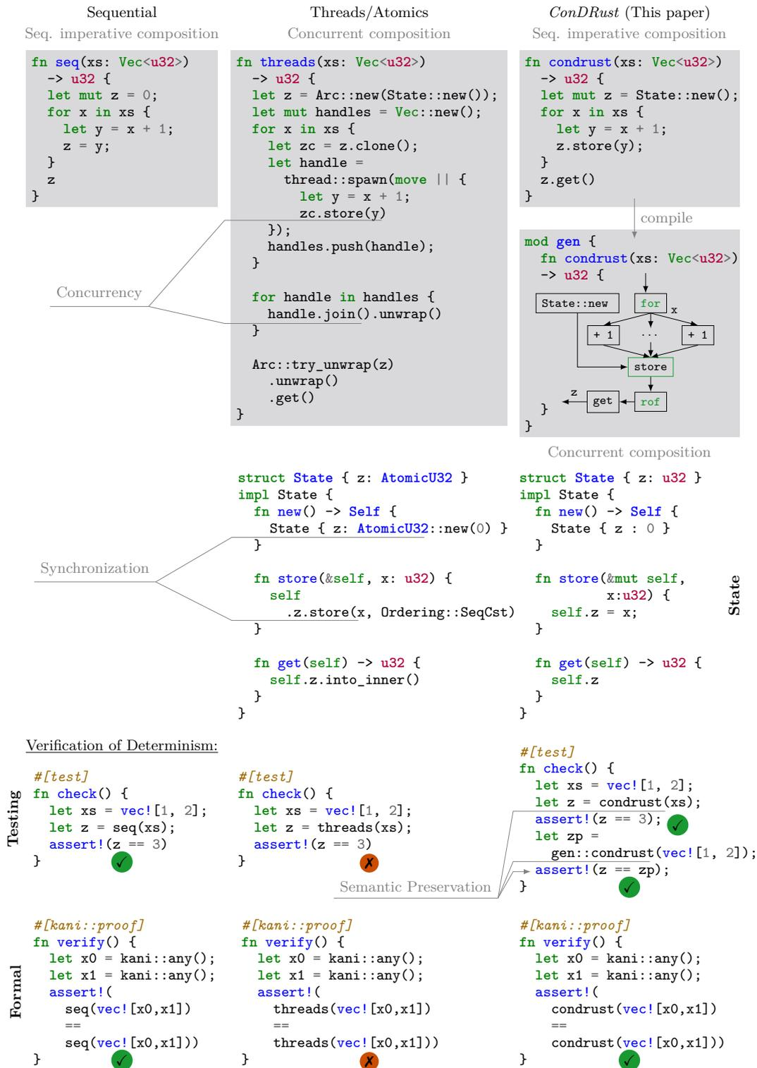
■ **Figure 2** Comparison between sequential, concurrent and *ConDRust* programs and their properties. The sequential program executes deterministically and is amenable to verification. The concurrent program offers parallel speedup but compromises determinism and verifiability. The *ConDRust* approach preserves determinism and verifiability and compiles the program into a concurrent dataflow for scalable parallel execution.
