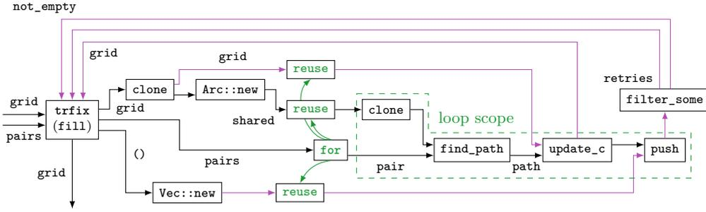
■ **Figure 7** *ConDRust* dataflow graph for the (unoptimized) labyrinth code listed in Figure 4. The graph contains *state arcs* that transfer state into and out of the *loop scope*. The *for* and *reuse* nodes make sure that processing inside the loop is well-balanced, i.e., does not get stuck.
