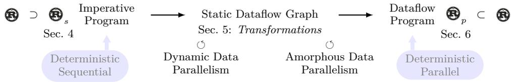
■ **Figure 1** The *ConDRust* compiler translates imperative programs written in  $\mathbb{R}_s$ , a subset of Rust for sequential composition, into dataflow programs in  $\mathbb{R}_p$ , a subset of Rust for parallel composition.
