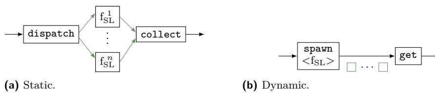
■ **Figure 9** Data parallelism inside a dataflow graph.
