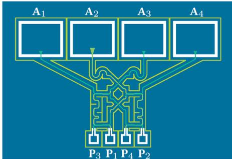
Fig. 6. Layout of Butler matrix with four input ports P (bottom) connecting a 1x4 antenna array of four patch antennas A (top).
