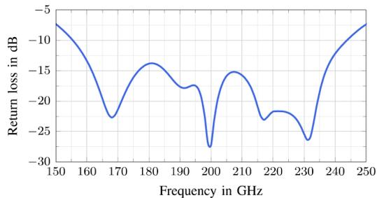
Fig. 5. Input reflection coefficient of antenna shown in Fig. 4 and further investigated in [9].
