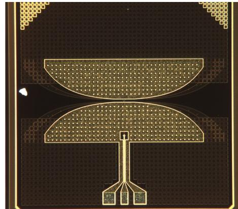
Fig. 4. Multiple stacked Vivaldi-shaped open slot antenna, fabricated in IHP SG13 process [10].
