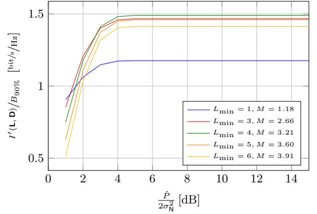
Fig. 2. Lower bound on the spectral efficiency for 1-bit quantized runlength modulated transmission with oversampling ratio  $M = \frac{1}{T_s B_{90\%}}$
