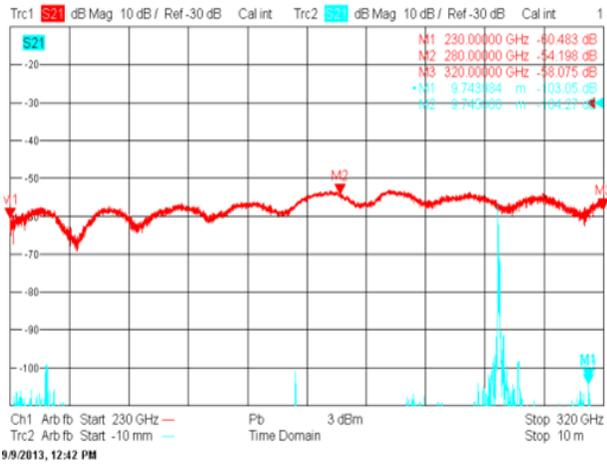
Fig. 3. Experiment setup (top) and impulse and frequency response after the reflection off wooden cabinet (bottom)
