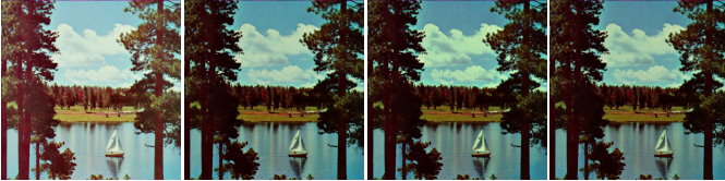
(a) Original image (b) Accurate (c) LeAp-5 (d) MBM [18] Fig. 4: PSNR of Image blending application computed with respect to the accurate multiplier-based filter: LeAp-5 PSNR=33.5, MBM [18] PSNR=32.6
